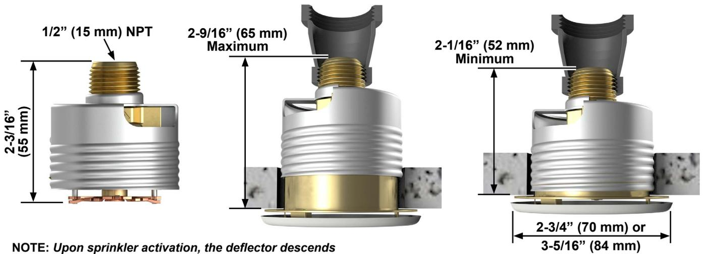
**NOTE:** Upon sprinkler activation, the deflector descends to approximately 13/16" (21 mm) below the sprinkler body.
